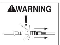
Always disconnect air from nailer whenever servicing! During maintenance, a nailer connected to air may fire accidentally, causing serious personal injury!
